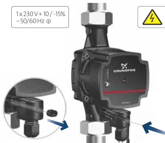
Fig. 17 Connecting the signal cable to the ALPHA1 L
